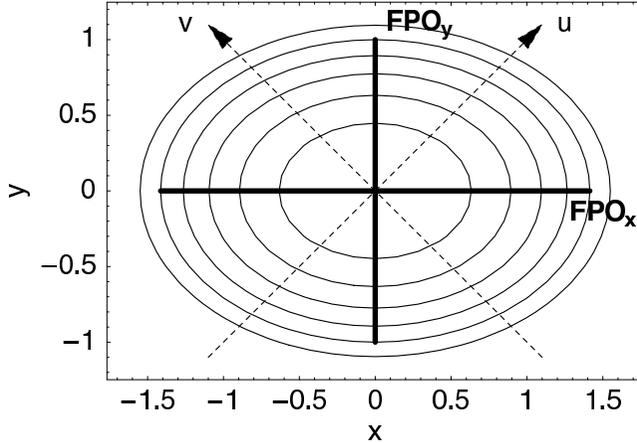
Fig. 2. Illustration of the two-dimensional harmonic oscillator (8) with  $\omega_x = 1$  and  $\omega_y = 2$ . Superimposed over the level lines of the potential energy are the FPOs in the  $x$  and  $y$  direction for  $E = 1$  (thick lines) and the rotated coordinate system (10). Both FPOs intersect the surface of section  $v = 0$  (which coincides with the  $u$ -axis) at  $u = 0$ .
